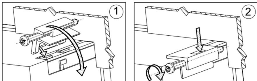
*Fig. 1. Controller fixing*
