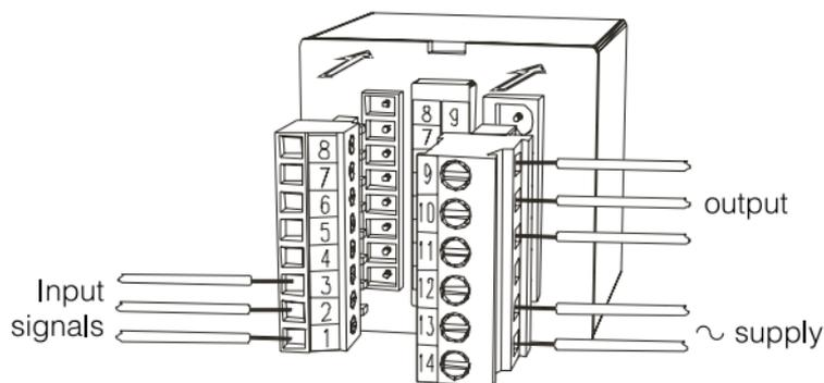
Fig. 3. View of controller connection strips.
