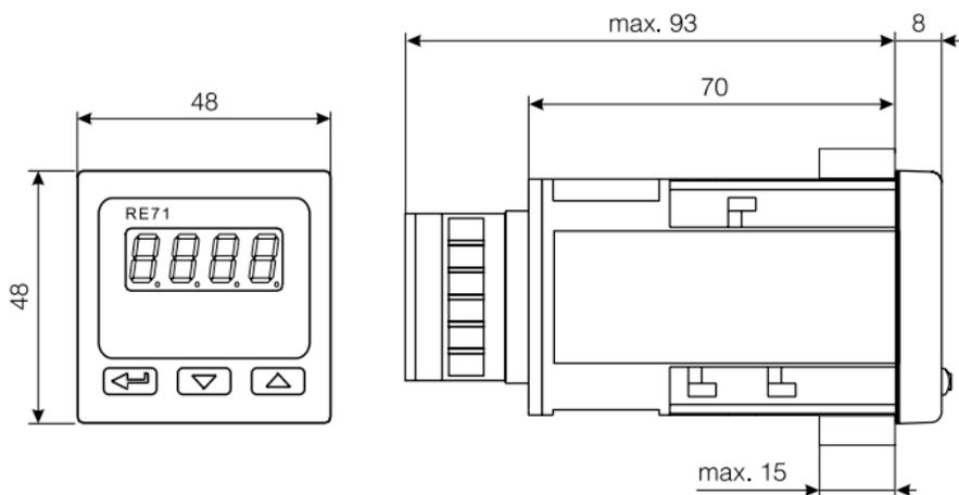
*Fig. 2. Controller overall dimensions*
