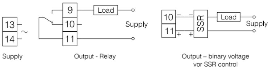
Fig. 5. Connection of the supply and load circuit.
