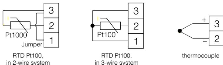
Fig. 4. Connection of input signals.
